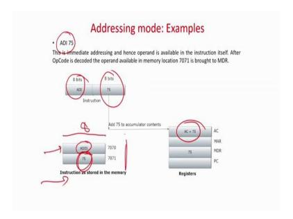
So, this is the first instruction is add immediate 75 so; that means, I told you it's a 8 bit as well as your data is also assumed to be 8 bits. Now in this case I told you the whole memory size is only 8 bits. So, the instruction this whole instruction together cannot fit into a single word add
